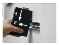
**Step 5:** Lightly press the button of DIN-Rail for remove it from the track.
