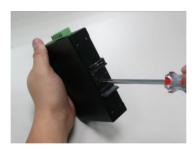
**Step 1:** screw the DIN-Rail on the Industrial 802.3at PoE Media Converter
