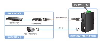
Figure 2-4: IGTP- 802T / IGTP-802TS Stand-alone Installation
