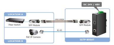
Figure 2-5: IGTP- 805AT Stand-alone Installation
